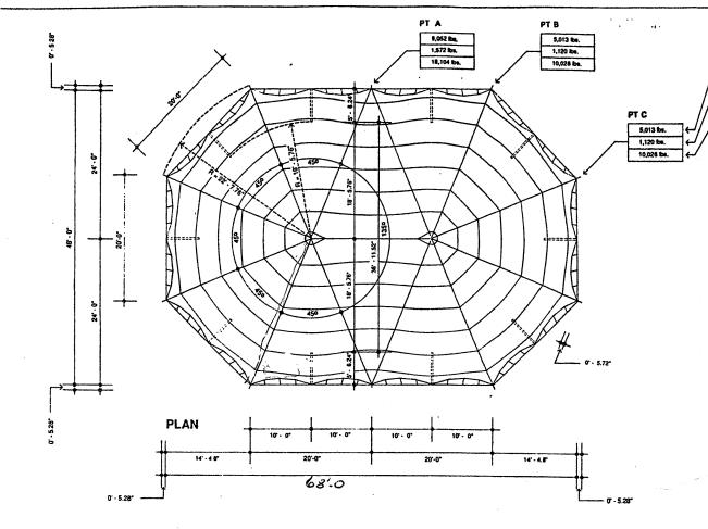
s umber represents the actual anchor link load anticipated under maximum design load. exerts the pre-stress force which is the amoun of tension necessary in the anchor link to properly pull the tent
